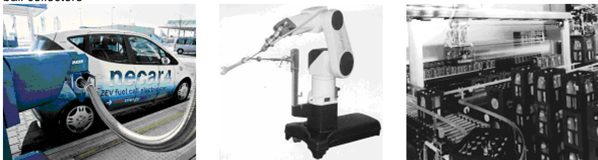
Service robot systems based on conventional robot arms: refueling, orthopedic surgery, automated drink terminal
